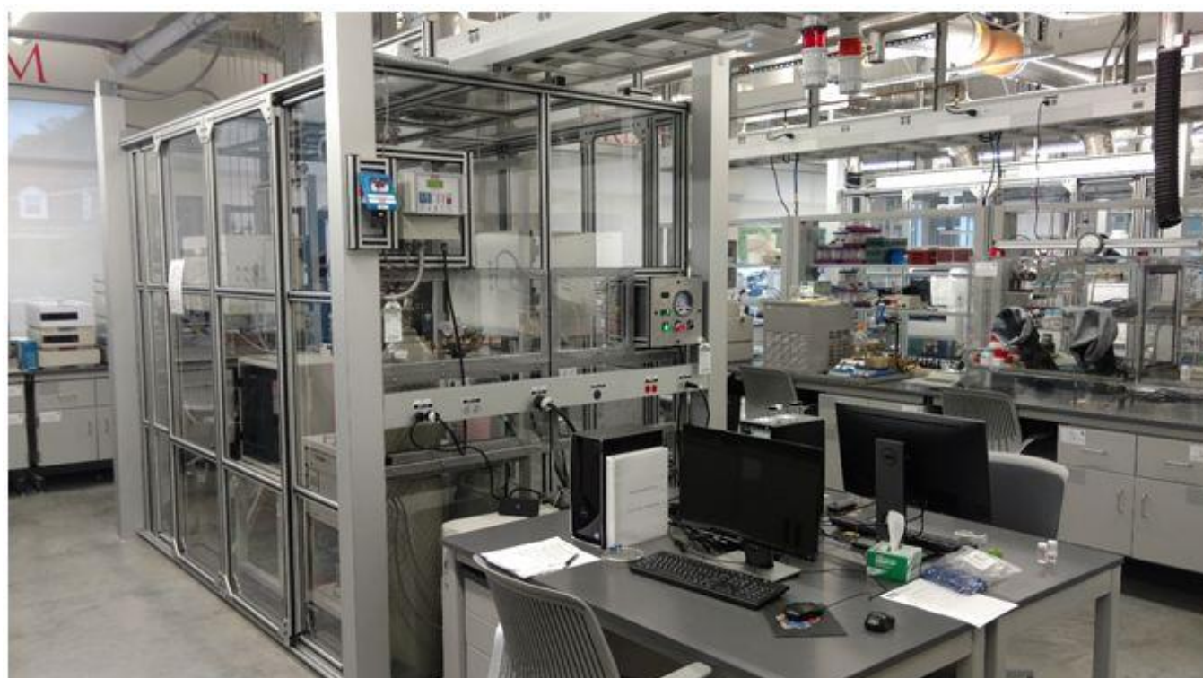
Figure 4 : Photo depicting the custom ventilated enclosure located at the south end of lab 2444. The dimensions (h x l x w) are 8 ft 10 inches x 10 ft x 5 ft 4 inches. The photo shows the attached gas detection system (front left), warning/alarm lights (top runner), interlock system (front right), colored outlets, safety equipment inspection tags, and PSM documentation (white folder next to computer tower).
