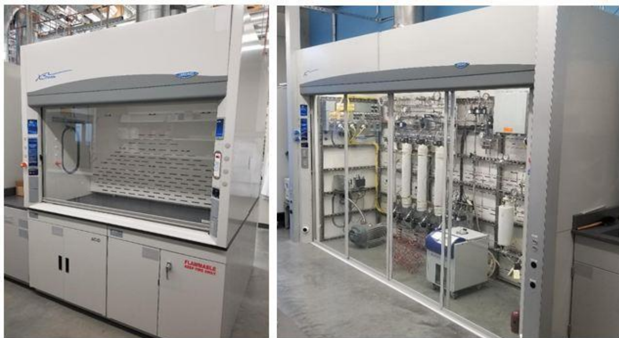
Figure 3: Labconco Chemical Fume Hood (left) with acid and flammable liquid storage cabinets located beneath the hood countertop, Labconco Floor Mounted Fume Hood (right).
