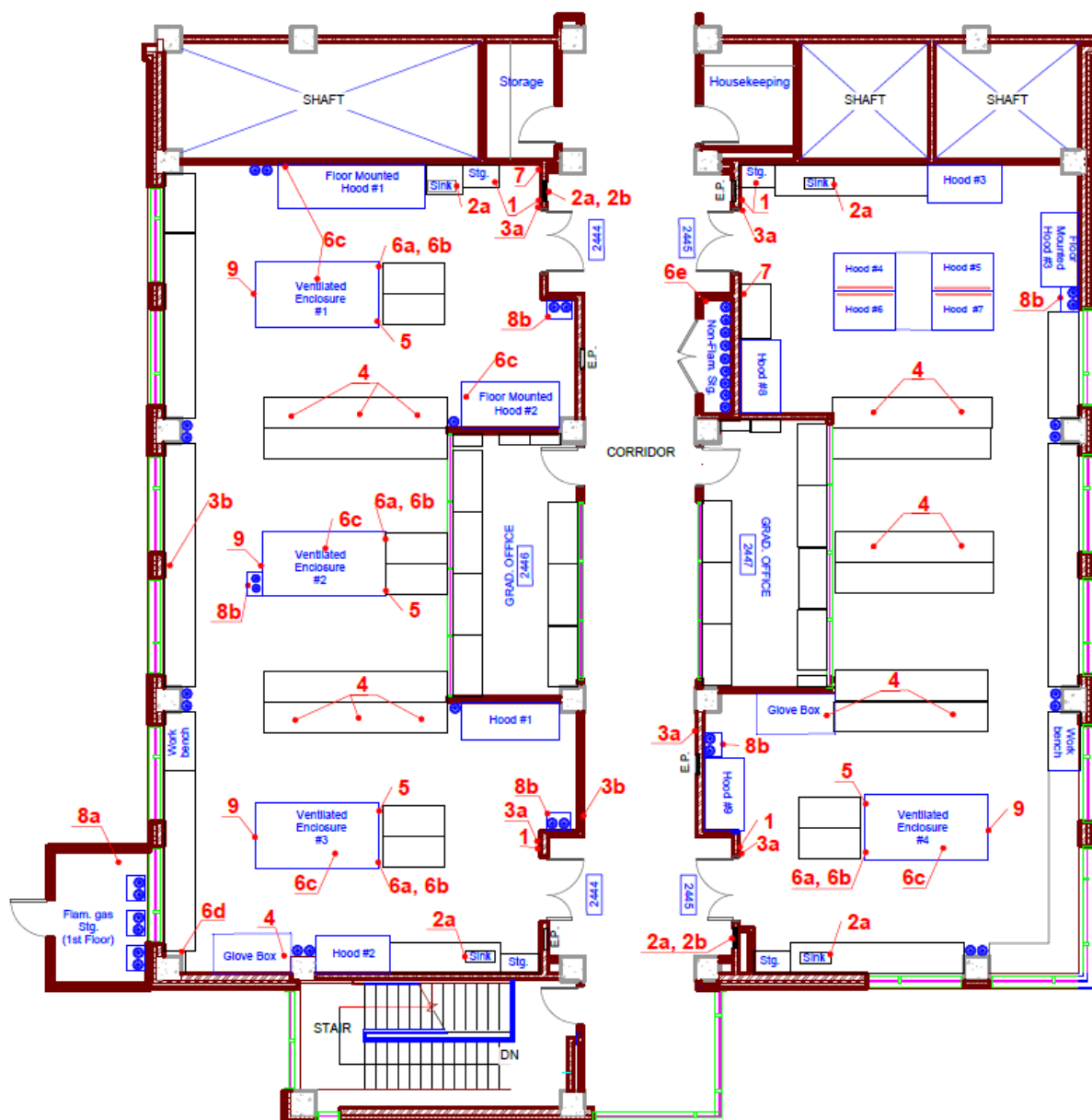
Figure 2 : Schematic of labs 2444 and 2445 and offices 2246 and 2247. Numbers designate the specific location of safety equipment located throughout the labs. General descriptions: Hoods, Ventilated Enclosures, Glove Boxes, and numbered items: 1. Personal Protective Equipment (PPE), 2. Eye wash and shower stations, 3. Fire extinguishers and fire alarms, 4. Ventilated dropdowns, 5. Interlock safety systems, 6. Gas detection systems, 7. Safety Data Sheet Compliance Center, 8. Ventilated cabinets, 9. Gas distribution panels. Numbers shown are referenced in the text.
