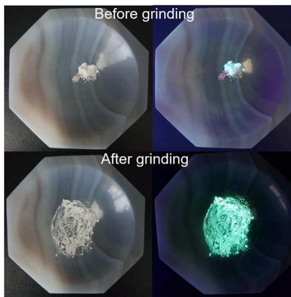
Figure 1. Photographs showing the three-component reactant mixture for compound 4 under ambient light (left) and UV light (right) before (top) and after grinding (bottom). Ligand L2 emits a weak blue color with \lambda_{em} = 460 nm in the solid state, which is distinctly different from the blue–green emission color of 4 ( \lambda_{em} = 504 nm)
