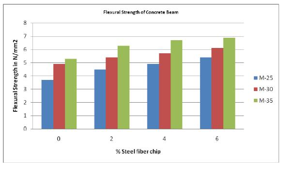
**Graph 4 – Flexural Strength of Concrete Beam**
