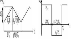
Fig (7.a) Inductor current waveform Fig (7.b) Inductor voltage waveform
