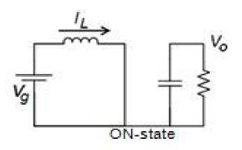
Fig (6) the ON state diagram of the boost converter.
