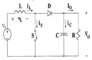
Fig 4 Circuit diagram of boost converter.
