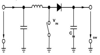
Fig 8 Boost Converter Power Stage.
