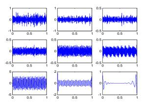
Fig.3 8Level DWT of vibration signal for healthy motor at full load
