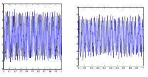
Fig.2 Vibration signal under full load for healthy and faulty motor respectively
