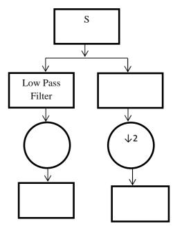
Fig.1 DWT decomposition of a signal
