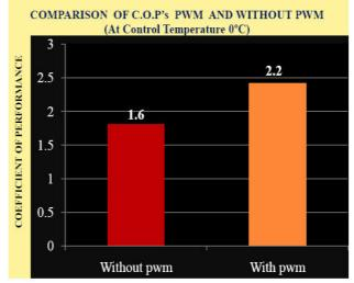
**5.** Comparison of coefficient of performance with and without pulse width modulation technique at control temperature  $-5^{\circ}$ C.
