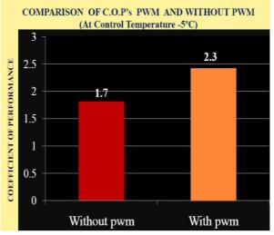
**6.** Comparison of coefficient of performance with and without pulse width modulation technique at control temperature  $-25^{\circ}$ C.
