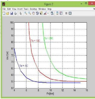
Fig.5. Condenser Fan power & Condenser Pressure
