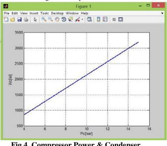
Fig.4. Compressor Power & Condenser Pressure
