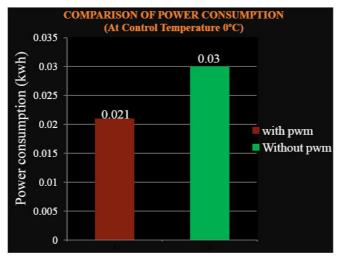
**2.** Comparison of power consumption with and without pulse width modulation technique at control temperature  $-5^{0}$ C.
