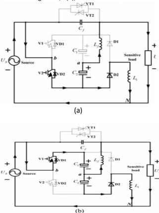
Fig.3. Operating conditions during positive halfcycle. (a) V2 switched on.(b) V2 switched off.
