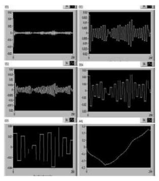
Figure 4: Detailed and approximate level coefficients level of Iq for healthy system.Experimental Setup: Setup consist of 3 H.P,
