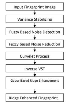
Fig 4: Block diagram for proposed system
