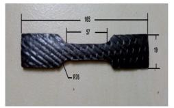
Figure 2: Sample Piece for Tensile Test (All dimensions are in mm)
