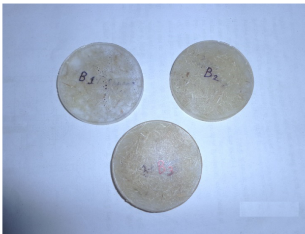
Fig. 2: Short banana fiber reinforced epoxy composites
