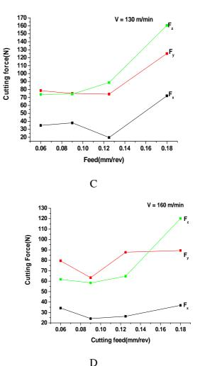
Fig. 2 Effect of speed on different forces (A, B, C, D)
