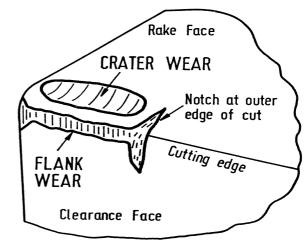
Fig. 1 Flank and crater wear
