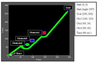
Fig. 7. Trajectory of the singlemobile robot with 3 obstacles
