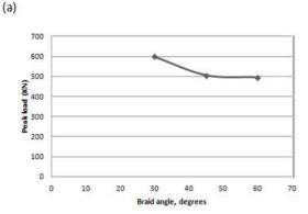
Fig. 10. (a). Variation in peak load with braid angle.
