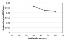
Fig. 19. (b). Variation in compressive strength with braid angle.
