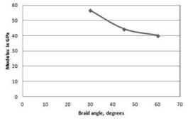
Fig. 8. Variation in modulus with braid angle.
