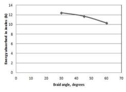
Fig. 9. (a). Variation in impact energy absorbed with braid angle.
