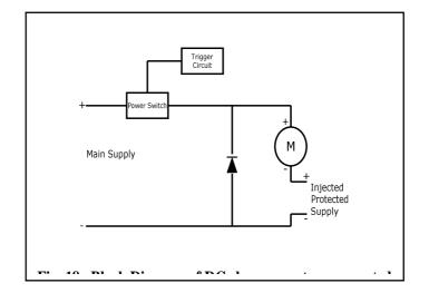
Fig. 18: Block diagram of the proposed DC chopper system
