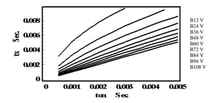
Fig. 17: The relationship between  $t_{on} \& t_x$  Vinj (battery) takes as a parameter.
