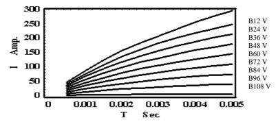
Fig. 16: The relationship between (Imax & ton), Vinj ( battery) takes as a parameter.
