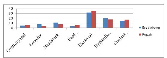
Fig. 1 CNC Lathe machine sub-system failure frequency and Downtime
