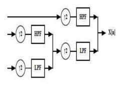
Figure 3. Wavelet reconstruction process.
