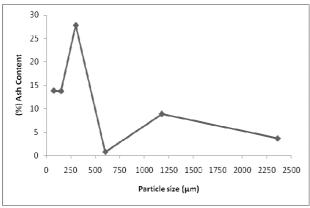
Fig 3: Effects of particle size on ash content of palm kernel shells
