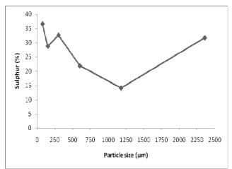
Fig 5: Effects of particle size on sulphur of palm kernel shells
