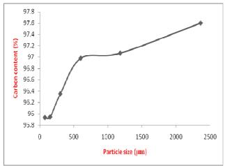
Fig 4: Effects of particle size on carbon content of palm kernel shells
