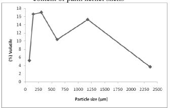
Fig 2: Effects of particle size on volatile content of palm kernel shells
