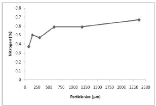
Fig 6: Effects of particle size on nitrogen of palm kernel shells
