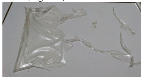
Fig. 1: Bioplastic from tapioca starch nanoparticle with ratio biopolymer : glycerol = 7:3.
