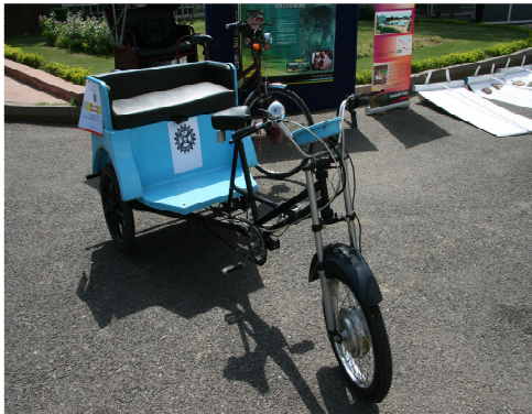
Fig 4-Solar Rickshaw by IMML with BLDC motor
